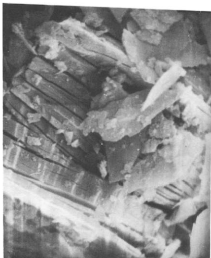
Fig. 6. Scanning electron micrograph of pandermite heated to 500°C. Original magnification 500×.
